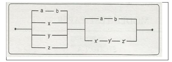
Using laws of Boolean algebra, simplify the circuit and construct an equivalent
